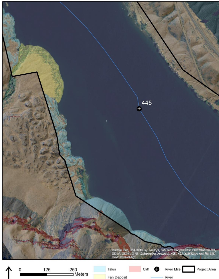
Figure 8. Detail map of project area near river mile 445. Areas classified as talus are light blue, fan deposits are yellow, and cliffs ( \geq 45^\circ ) are red. Image overlaid with LiDAR derived hillshade. Aerial imagery provided by ESRI (2017b).
